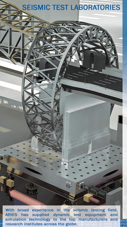
ARIES Seismic Simulation Systems accurately reproduce true earthquake conditions, allowing civil engineering researchers to evaluate the behaviour of any test specimen, from small structural components full-scale structures, under these excitation conditions.
